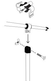
5. Assemble the top horizontal tube with joint locks. See instructions on top horizontal tube. Be sure to mount the top horizontal tube at the marking on the joint lock.
