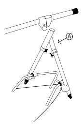
Make sure the tap in the T-connector fits the hole in the 35 mm tube.
