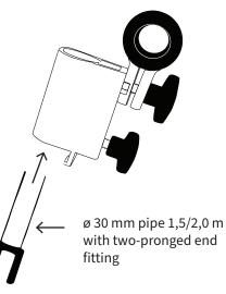
If your boat is wide in the stern, mount the pulpit connectors in front or rear portion of the push-pit.
