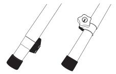
3. Mount the plastic plugs on two of the top horizontal tubes.
