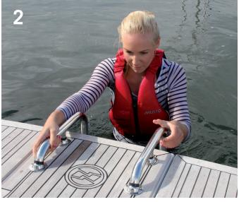
2. DEPTH The ladder should be extendible at least two steps below the water to easily be able to climb up the ladder.
