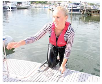
4. ALL THE WAY There should be grips and steps to get all the way into the boat, not only out of the water.
