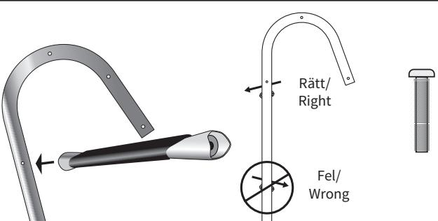
Attach the footsteps to this stay (on the inside). Make sure that the step angle is correct - they should slope upwards when you climb.
