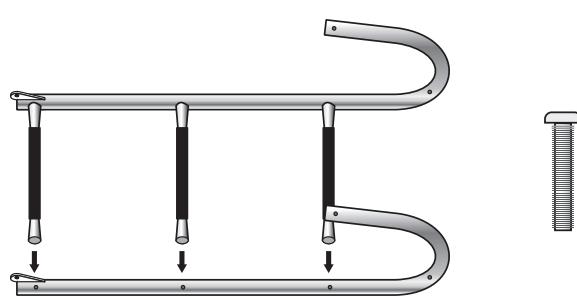
Assemble the second curved strut in the step. /
