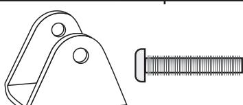
U-brackets are attached to the steps. These and those on the struts are attached to the hull with acid-proof bolts of a suitable size (not included). /
