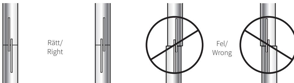
Check the fit with the lower part at the hinges first so that the steps are mounted on the right side of the curved strut.
