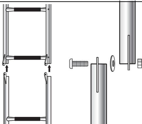
Assemble the upper and lower part of the steps at the hinges. /
