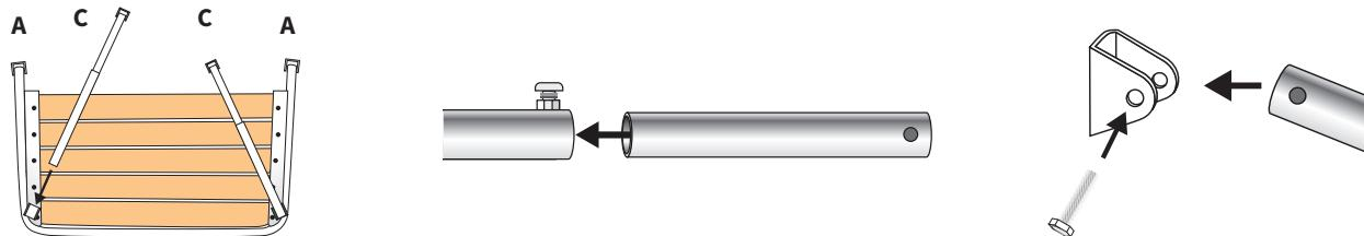
Check that all parts are included. Install the strut. Attach the u-brackets so that they can be adjusted against the hull.
