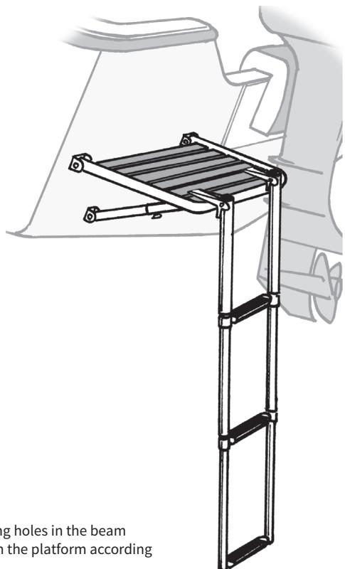
The ladder is attached to the existing beam under the teak. Drill holes in the teak through the existing holes in the beam before mounting with bolts. Suitable ladder for the bathing platform (extra equipment). Mounted on the platform according to the pictures above. /
