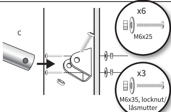
Drill holes in the hull for the u-bracket and screw them in (unclip them from the platform first). Attach the platform to the u-bracket. /
